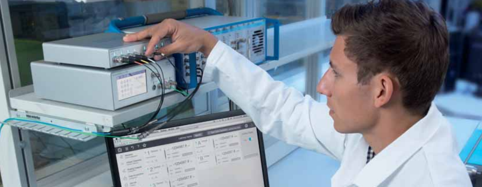
Charge amplifier calibration with a precision calibrator
